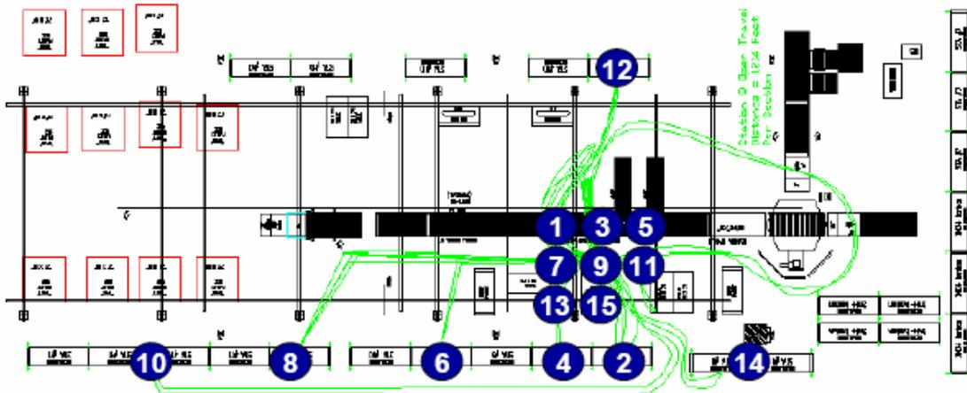
Value Stream Mapping (VSM) and spaghetti diagramming are often used in conjunction with each other. The object of utilizing VSM is to eliminate wasted time and handling associated with the issuing, receiving and storage of inventory.
